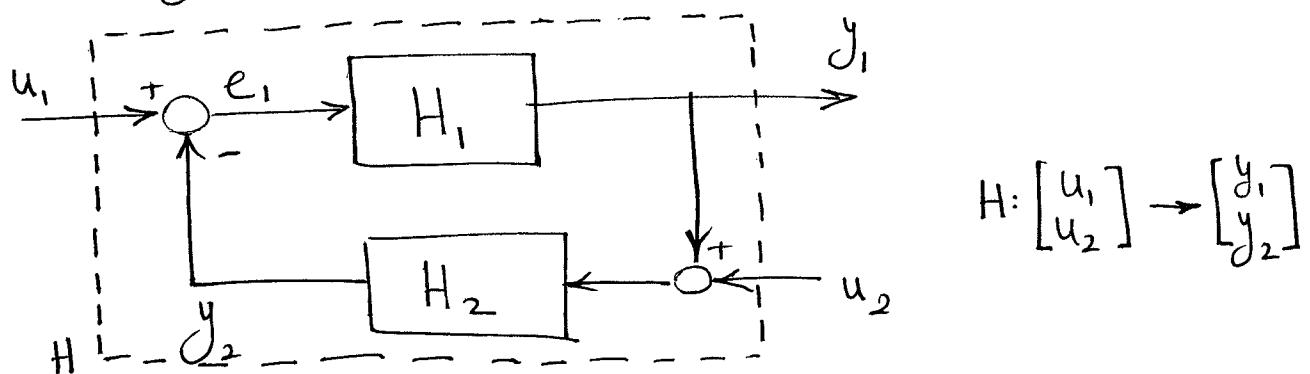
a)  $H_i$ : passive with storage functions  $V_i$  &  $V_{\bar{i}}$
