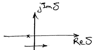
Supercritical Hopf bifurcation involves loss of stability of an e.p. which is stable focus and formulation of a stable limit cycle.
