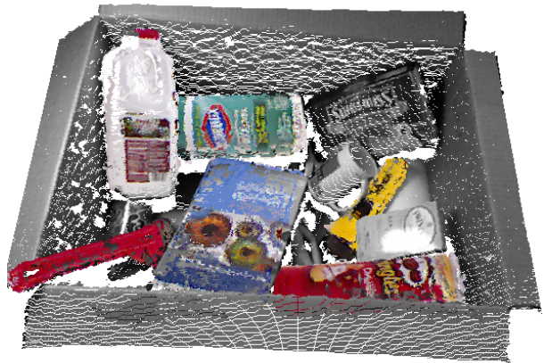
Fig. 1. Overview. Our approach exploits both geometric shape and color information in point clouds for robust object pose estimation. The estimated pose of each object is depicted in color object point cloud. Since our approach does not hinge upon the planar segmentation, it can be applied in highly cluttered environment. (Best viewed in color)
