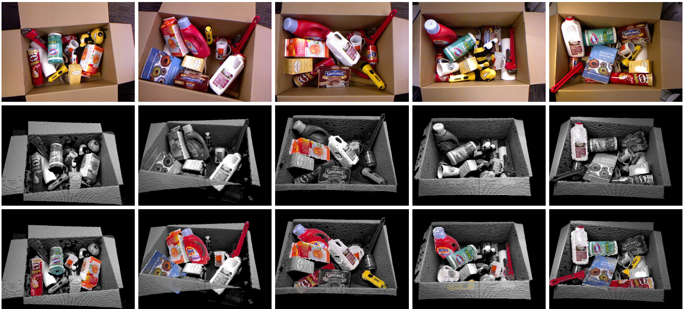
Fig. 7. Selected pose estimation results of Drost et al. [21] (second row) and our approach (third row). The first row shows the color image of scanned scenes. Correct pose estimates are depicted in color point clouds in second and third rows. In cluttered scenes, [21] works poorly because the low dimensional PPF feature does not give good matches between the model and the scene. Using the color information, CPPF is more discriminative so that pose results from the voting scheme result in the true positive poses. (Best viewed in color)
