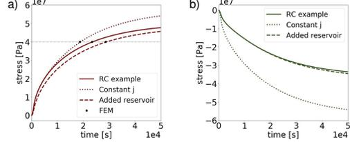
Fig. 6. SPICE results at a)  $x = 0$  (cathode) and b)  $x = L$  (anode) for our example of a two-segment wire, the case with constant current density  $j$  for the whole wire for comparison, and our example with a reservoir added to the cathode end at  $x = 0$ . The stress axis corresponds to the voltage results from the simulation. The results fit well with FEM, the points marked with dots are the FEM lifetime results.
