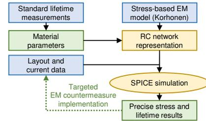
Fig. 1. Overview of our proposed flow on how to apply stress-based EM modeling in IC design. Blue boxes correspond to existing data and models, yellow boxes to recent EM modeling methods, and green boxes highlight the contributions of this paper.
